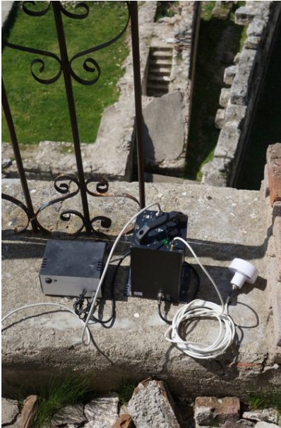
Ambient vibration test equipment on the roof, 2016
