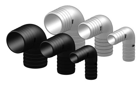
Tru-Design Connectors are moulded from a glass reinforced nylon composite. High strength, high-modulus glass fibres impregnated into the nylon provides dramatic strength, stiffness, toughness, and dimensional stability.
